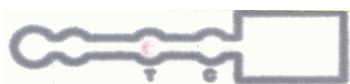
Figure 8 – Capture of RNA target stand by a complementary strand in the presence of CBM64-ZZ:anti-biotin antibody complex in paper microfluidic channels. The reaction mixture migrates across the channel with the aid of a running buffer (PBS 1%, BSA 0.5%, Tween 0.01%, Saccharose 2.5%).
